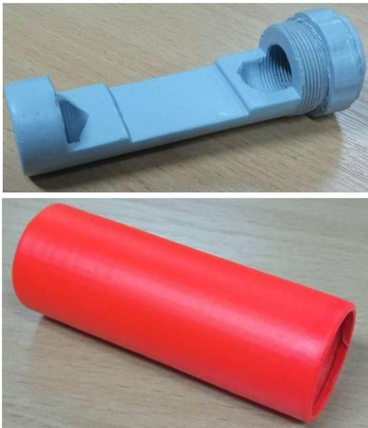
Figure 8: Additional mechanical processing-gritting and final polishing P1000
