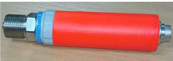
Figure 9: Realized small electronics enclosure for pressure transmitter
